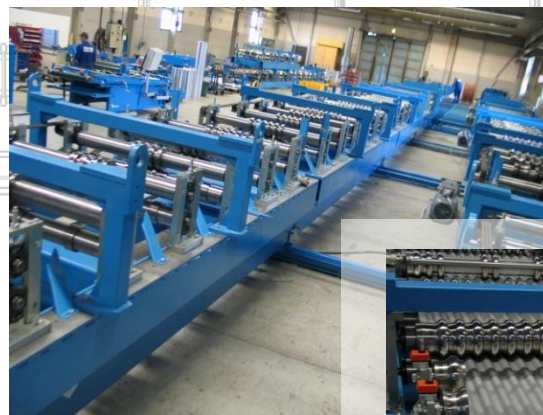
Rollforming cassettes & base frames
