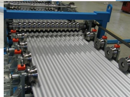
Rollforming cassettes & base frames
