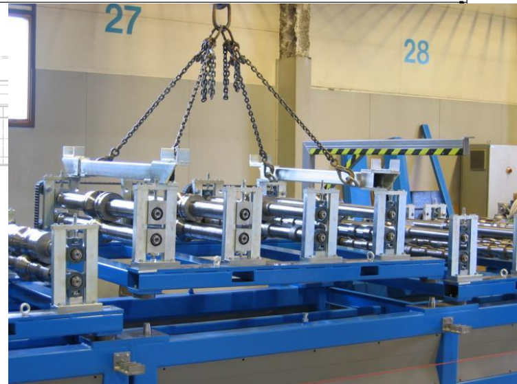
Rollforming Tools in Quick-Change Cassettes
