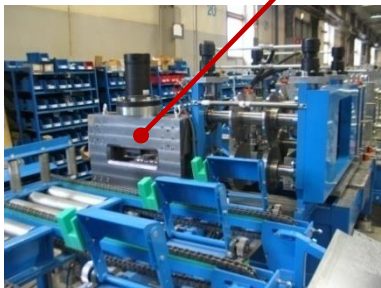
END TAB BENDING UNIT
