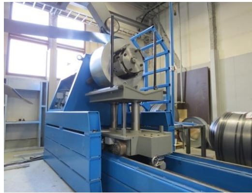
DECOILER & COIL CAR
