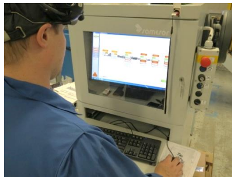
LINE CONTROL WORKSTATION (PC) Line control, order queue handling, interfacing, data storing etc.
